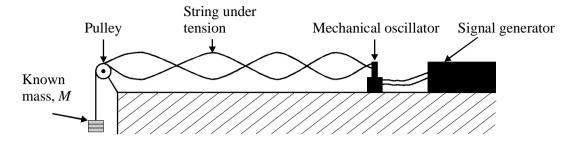
For a particular mass, the student adjusts the frequency f of the signal generator until a standing wave is established. The frequency f and the wavelength  $\lambda$  are recorded. The procedure is repeated for a range of masses.
